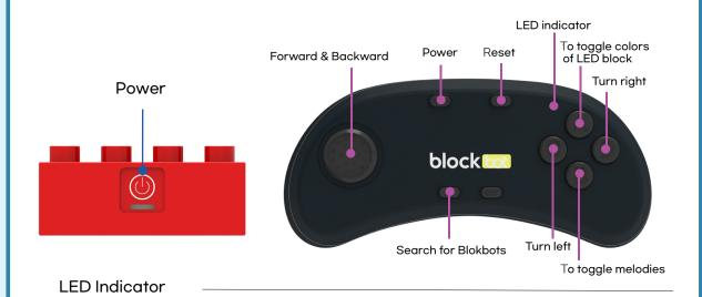
Blue: Looking for Blockbots to connect. Green: Connection established. Red: Failed to locate a Blockbot. If LED alternates RED & Green, please change battery of remote.
